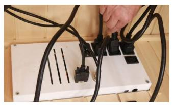
Plug in all heater leads to the receptacles on top of the power supply box.
