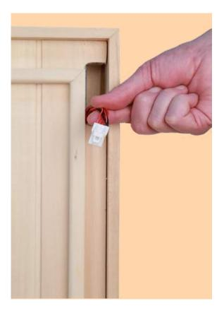
Pull the single plastic connector down and out of the roof before lifting the roof into place. If you are unable to grab hold of the connector through the small opening in the ceiling, it may be necessary to remove the first T&G board on the top left side of the roof and feed the connector down through the opening.
