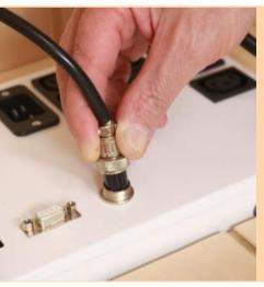
Connect the circular connector to power supply box. Align the groove in connector to properly insert.
