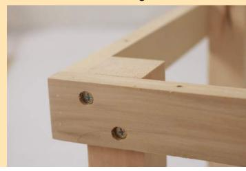
Attach the leg assembly to the bottom of the bench surface. Choose which surface of the bench you prefer to be the top and bottom.
